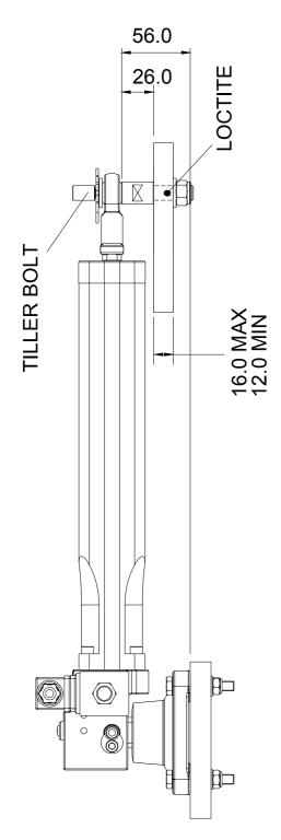
The tiller bolt supplied is suitable for a quadrant thickness of 12 to 16mm.
