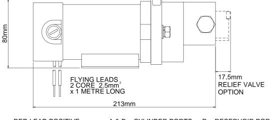
RED LEAD POSITIVE -PRESSURE TO 'A' PORT A & B = CYLINDER PORTS G1/4 (BSP) PARALLEL R = RESERVOIR PORT G1/4 (BSP) PARALLEL
